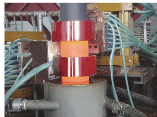
轧辊双频淬火 Dual Frequency Hardening for Roller
